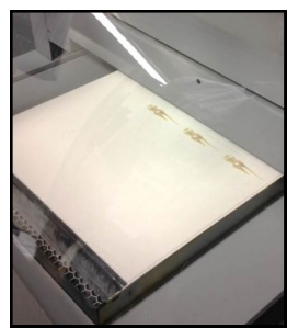
Print in progress in the build envelope
